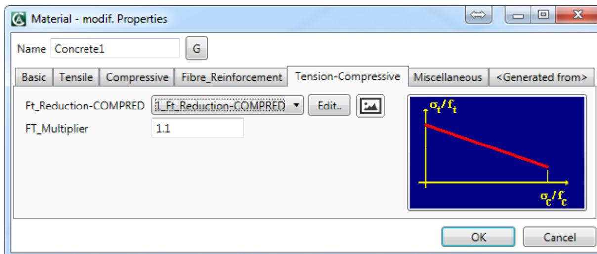
Fig. 2-37: Dialog Concrete SHCC – Tension-Compressive parameters
