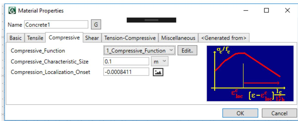
Fig. 2-29: Dialog Concrete User – Compressive parameters
