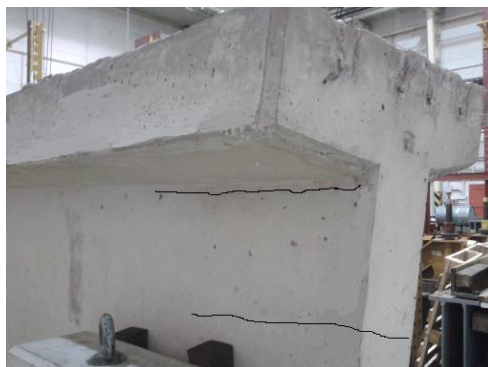
Figure 12: Spalling crack in the end of the beam
