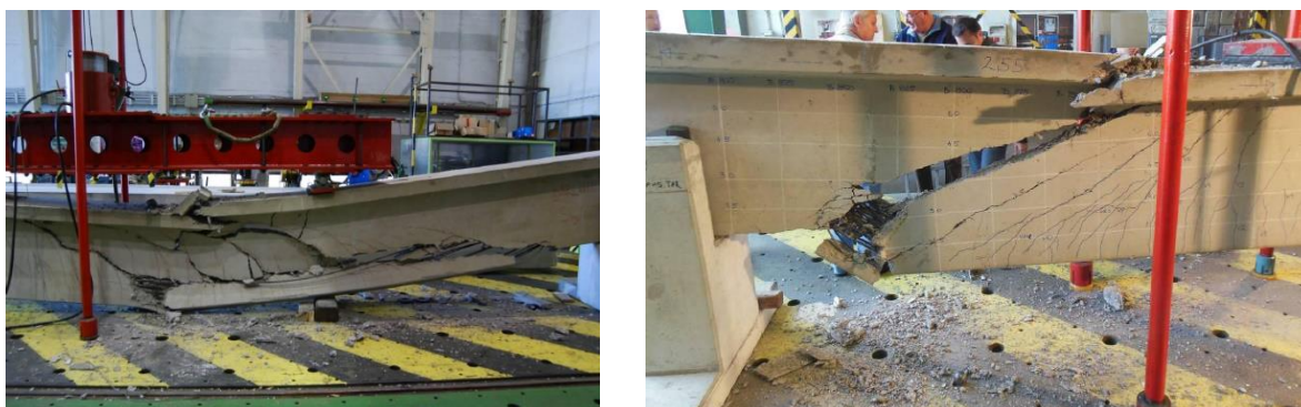
Figure 15: Bending (left) and shear (right) tests
