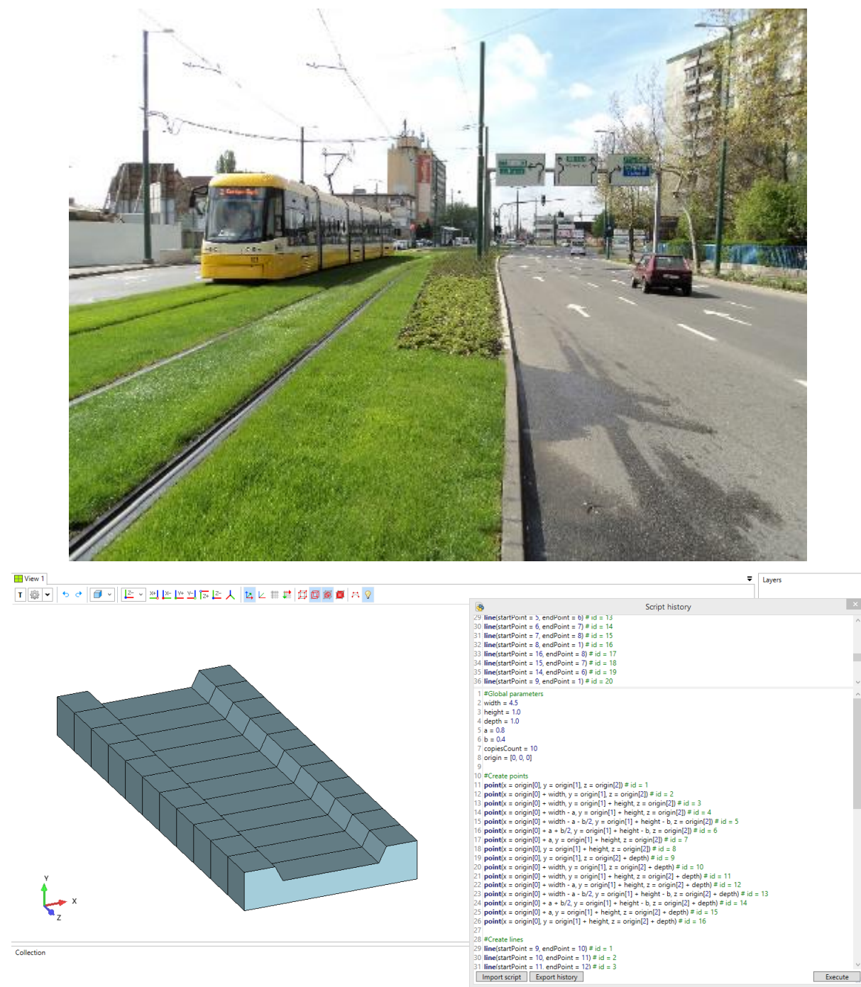
Fig. 6: Example of parametric script for generating rails. Solid view
