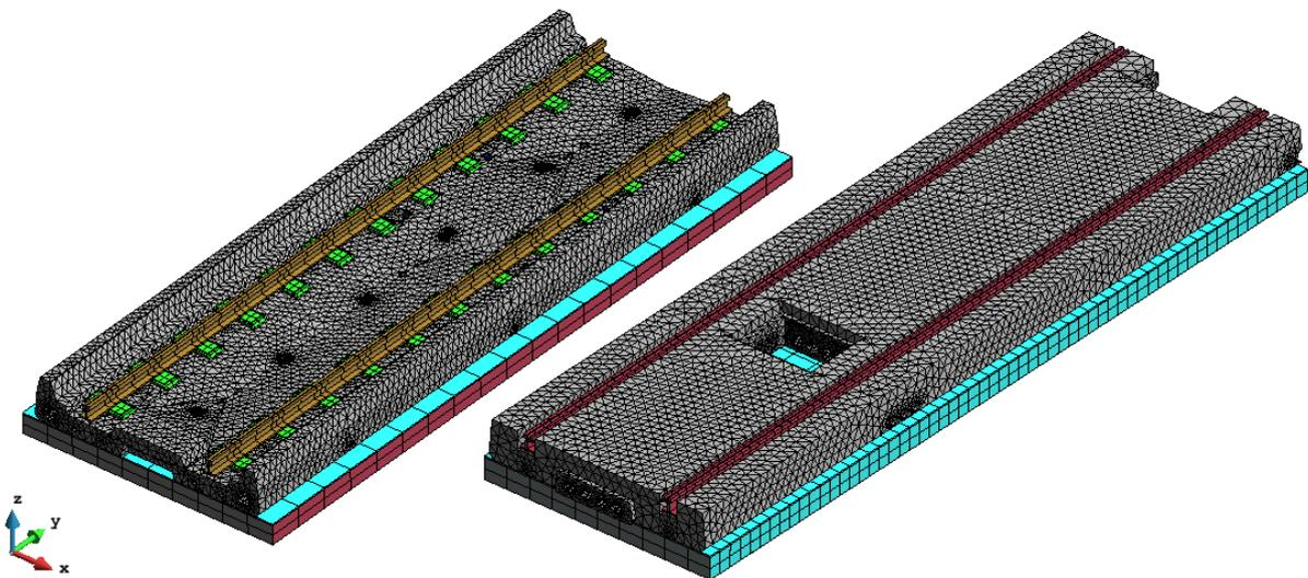
Fig. 2 Numerical models of the precast slabs
