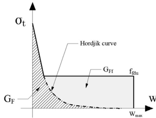
Fig. 4 Used tensile function for numerical calculation
